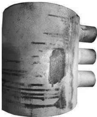
Fig. 3. The specimen for metallographic replica
