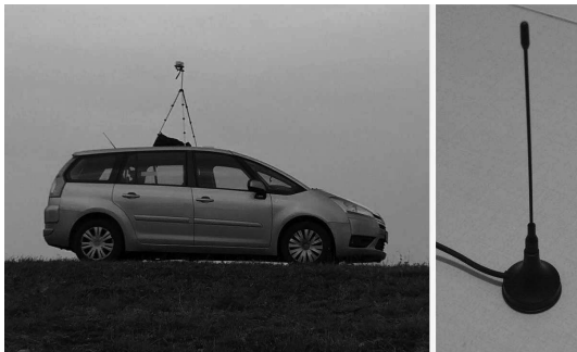
Fig. 6. Fixed node MP1(left), GSM antenna (right)
