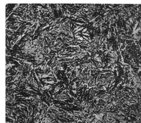
Fig. 5. High-grade martensite in steel microstructure (amplification 500x) [4]
