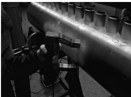
Fig. 2. MT examination of 13CrMo4-5 the headers
