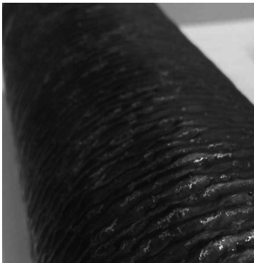
Fig. 6. Sample overlay welded in protection of two-component gas mixture
