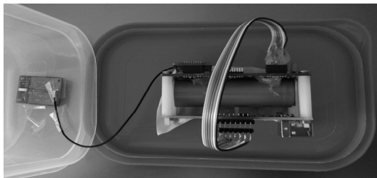
Fig. 1. LPWAN node with Chip antenna and USB connection for the PC
