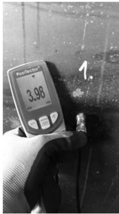
Fig. 4. Measurement of the thickness of the wall
