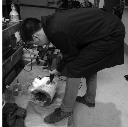
Fig. 4. The principle of applying the replicas
