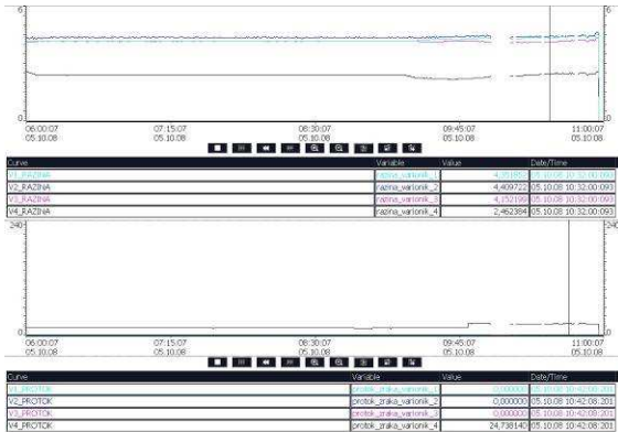
Fig. 7. Measurement historical data representation for vessels levels in meters (upper graph) and flow of air in fermenters in \text{m}^3 in hour (lower graph) (color inverted)
