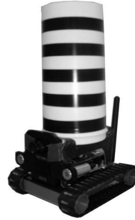
Fig. 4. Surveyor SRV1 robot with the zebra pattern
