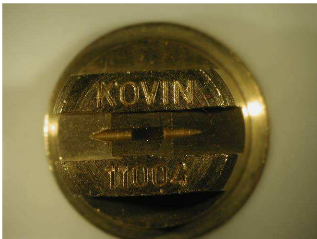
Figure 2. The nozzle 11004 tags made of brass company by "Mlaz" and "Kovin"
