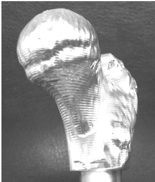
Figure 6. Final shape of the machined hip bone
