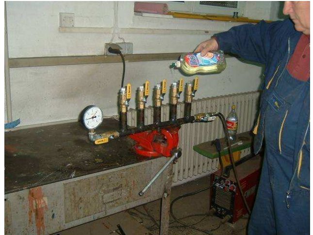
Fig. 7. Testing joints tightness [3]
