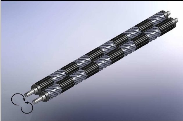
Fig. 14 Couple (pair) second variant husker roll
