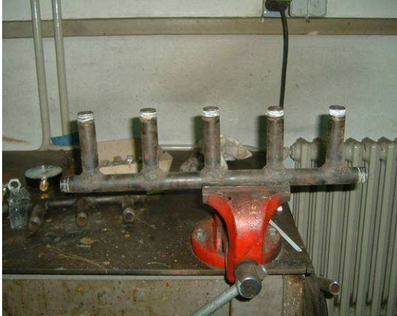
Fig. 6. Prepared test tubes with sealing cord Loctite 55 [3]
