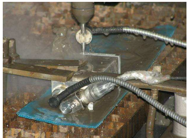
Figure.1 Diagnostic measuring vibration during cutting aluminium
