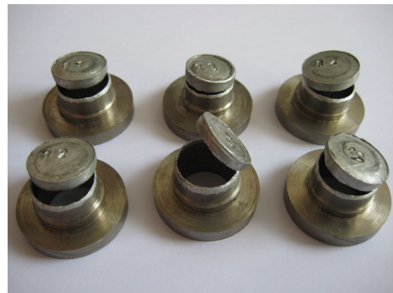
Fig. 2. Specimens after tensile test
