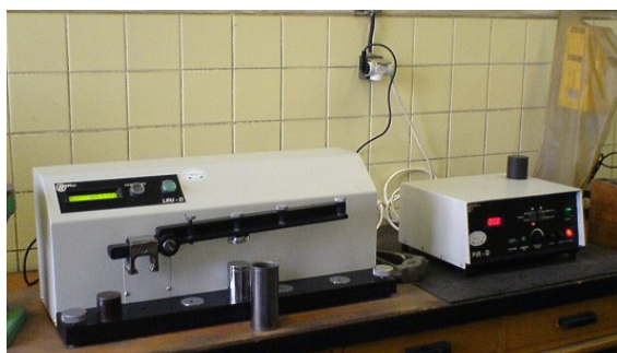
Fig. 1. Devices for moulding material strength properties measurement LRU-D and permeability measurement LPiR-D [3]
