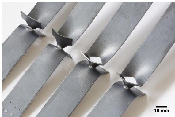
Fig. 3. Overall look on specimen No. 7 after the shear test
