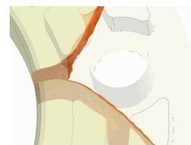
Fig. 6. Weld line formation
