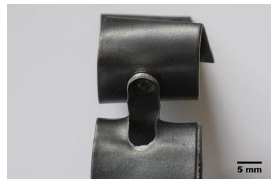
Fig. 1. Specimen No. 7 after the peel test
