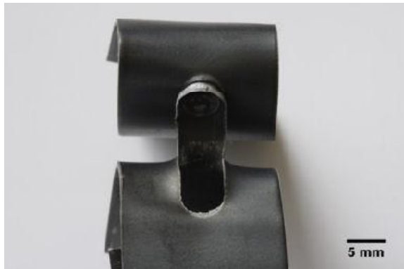
Fig. 2. Specimen No. 10 after the peel test
