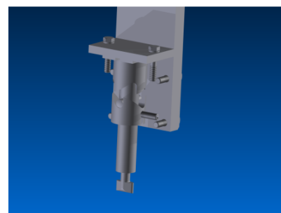
Fig. 10. Mechanism for automated opening/closing of lever arms
