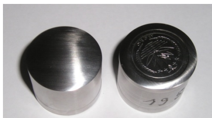
Fig. 2. Rollers prior to measurement of stress
