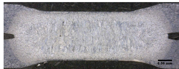
Fig..5. Macrostructure of joint (specimen No. 7)
