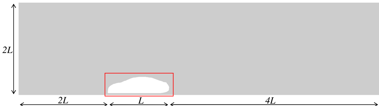
Figure 4: Dimensions and discretization of 2D domain
