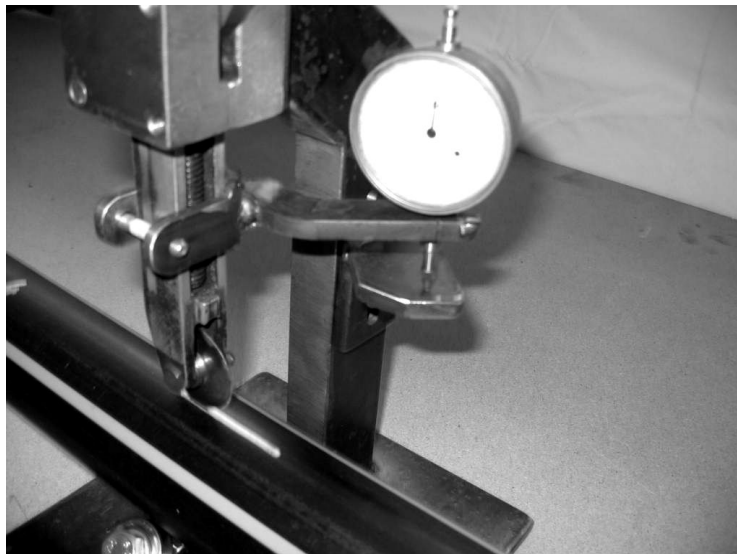
Figure 1b): Device for cutting of an initial radial notch [8,9]
