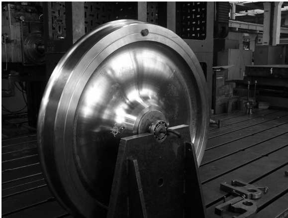
Figure 7: Static Wheel balancing
