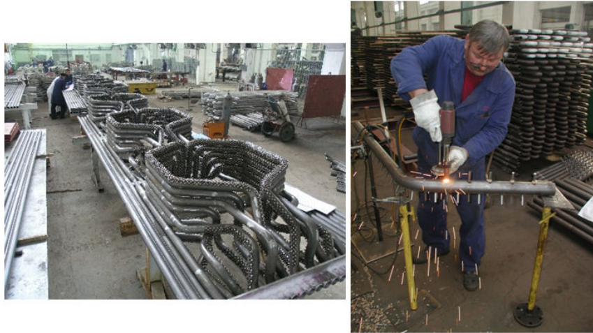
Figure 9. An example of manual stud arc welding in steam boiler production
