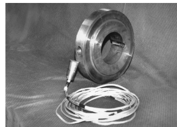
Figure 4. Thermocouple pin assembled and prepared for installation in the experimental ring
