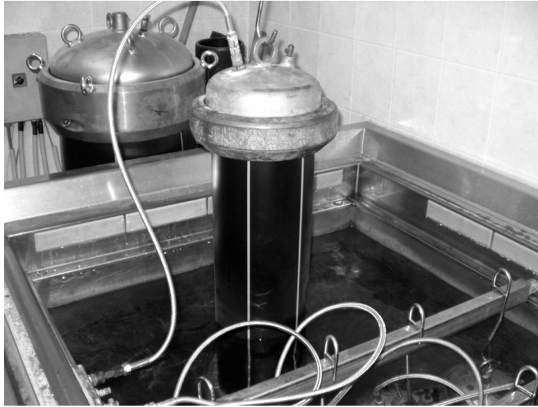
Figure 2: Mounting of pipe specimen into hot water tank [8,9]
