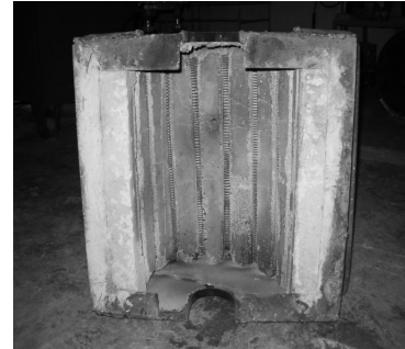
Figure 6. The setting of loops inside the electrical furnace
