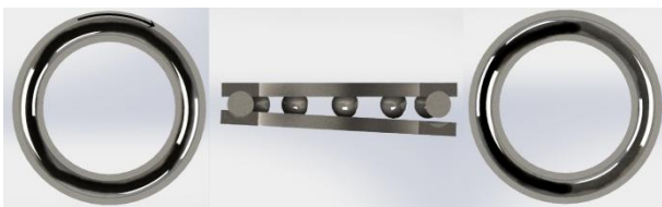
Figure 2.14 Housing washer misaligned
