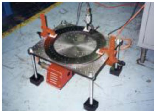
Figure 4.2 Use of the 2A inductor for surface protection under the coupling [2]
