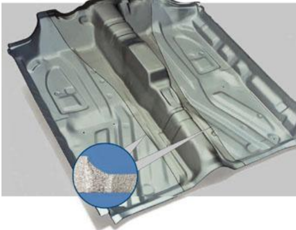
Figure 3. Floor panel of the car, formed from tailored sheet
