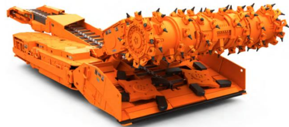
Figure 1. (a) conical pick; (b) continuous miner machine with fitted conical picks (courtesy: joyglobal) [22]
