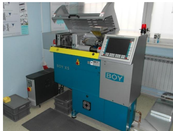
Figure 1. Injection molding machine installed at Mechanical engineering faculty in Slavonski Brod
