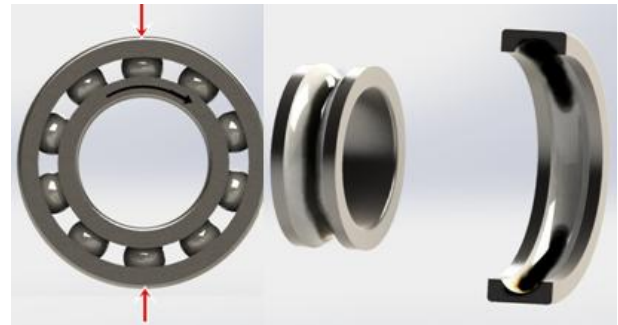
Figure 2.10 Oval compression of outer ring
