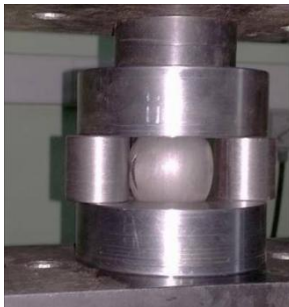
Figure 2. Tube expanding up to breaking
