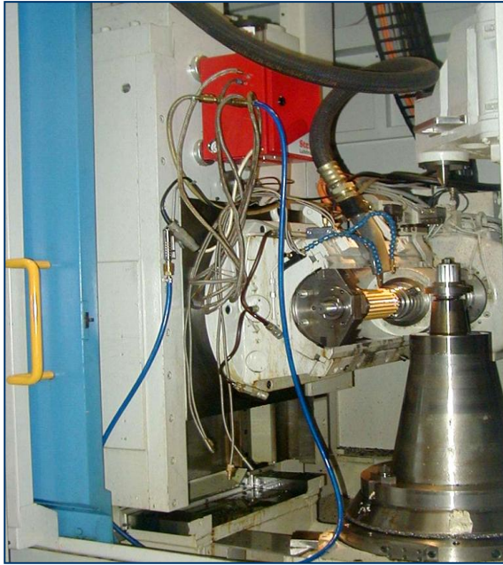
Figure 21. Environmental lubricant devices on Phauter PE-500 CNC milling machine.
