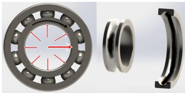
Figure 2.3 Radial load rotating in phase with the inner ring
