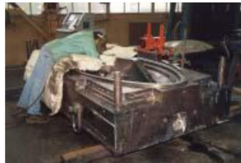
Figure 4.4 Application of vibro device during welding [2]
