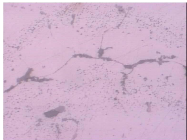
Figure 4. Pearlite at grain boundaries (x725)
