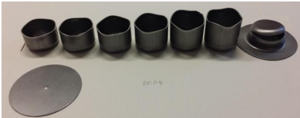
Figure 3. Initial blank and drawn cups of DC04
