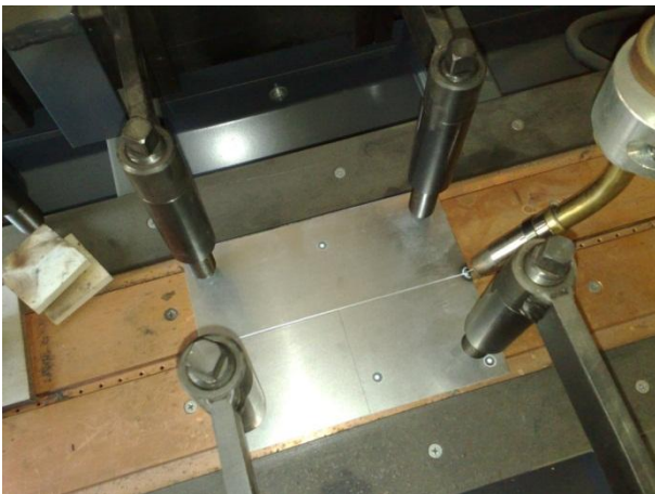
Figure 5. Fixation of materials prior to automated GMAW
