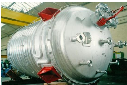
Figure 1. Pressure vessel made of DSS [2]
