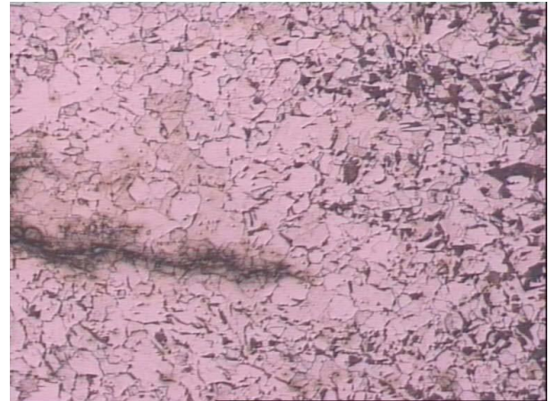
Figure 3. Crack-decarburation detail around crack (x75)
