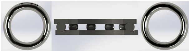
Figure 2.13 Housing washer positioned eccentrically relative to shaft washer
