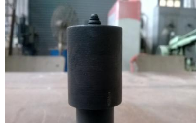
Figure 3. FSW tool with threaded pin
