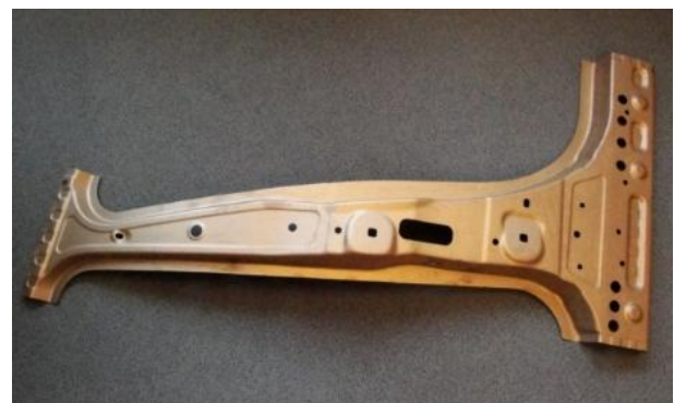
Figure 2. “B” pillar of the car made from tailored blank
