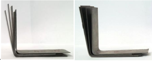
Figure 5. Bent part from homogeneous steel sheets with bending radius 3(left) and 5m too.
