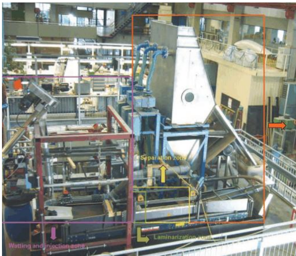
Figure 4. Magnetohydrostatic separator built-up in the EU7 project W2Plastics at Delft University, Holland
