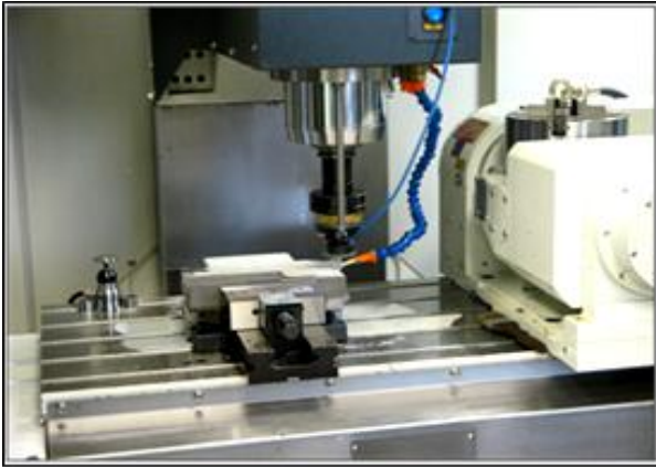
Figure 4.1. Work place with force and torque measuring system
