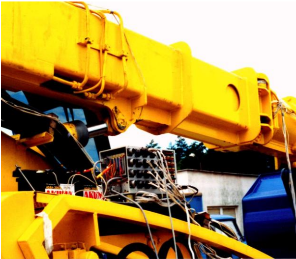
Figure 3. Data Logging and Processing Equipment
