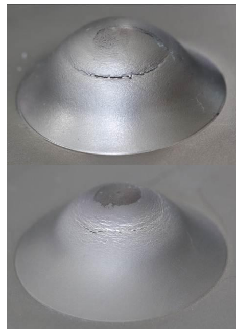
Figure 4 Erichsen cupping test: DC 01 (top) and PLASOX process (bottom)
