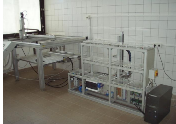
Figure 1. Flexible assembly cell with shelf storage.
