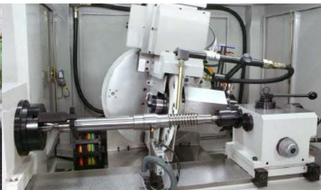
Figure 1b. Work zone of a grinding machine for machining of short threaded profiles
