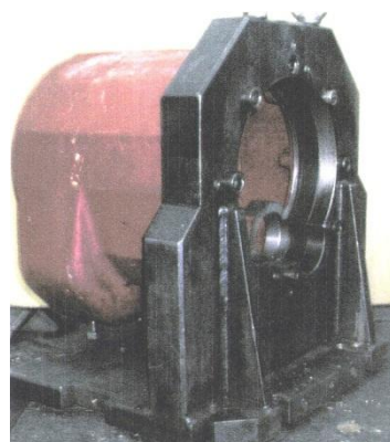
Figure 10 The realised fixture for the main clamping with the workpiece
