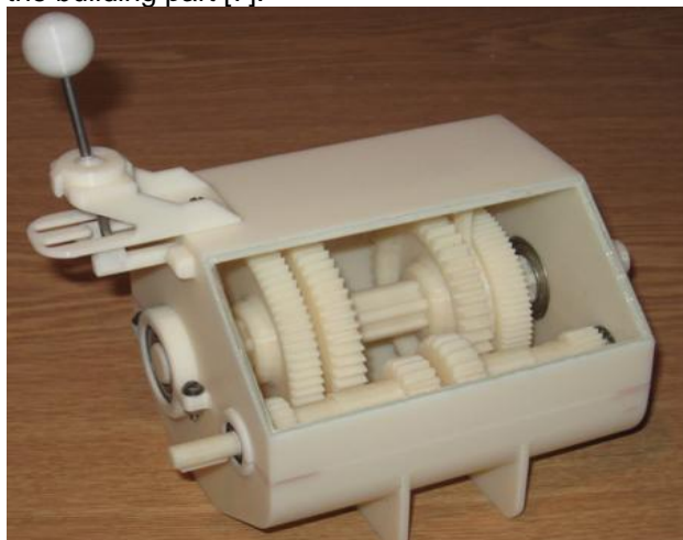
Figure 6. Assembled prototype of FDM gearbox
