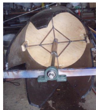
Figure 3. Installation of reinforcement and centring the front part
