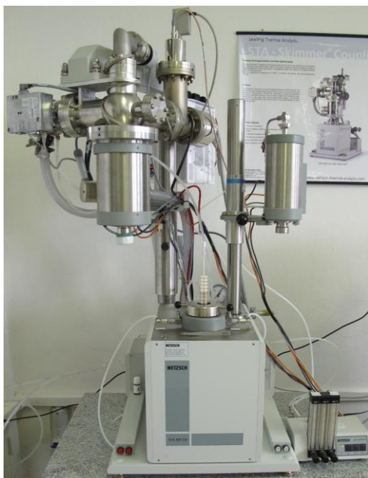
Figure 1. Netzsch STA 409CD – Simultaneous Thermal Analysis Apparatus
