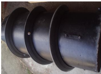
Figure 4. Adhesion of rubber profile
