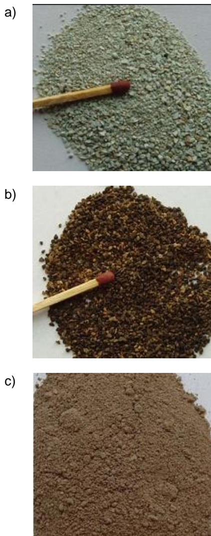
Figure 2 Klinopur – Mn a) original; b) after contact filtration; c) after contact filtration - crushed
