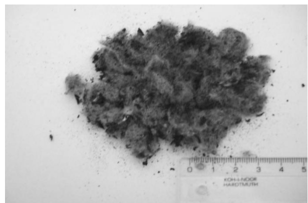
Figure 1. Fabric from used tires [4].
