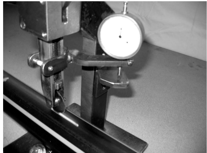
Fig. 1b). Device for cutting of an initial radial notch [8,9]
