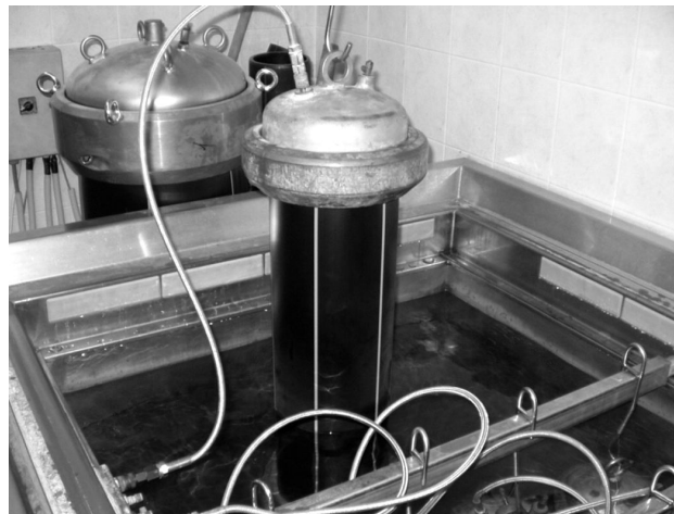
Fig. 2. Mounting of pipe specimen into hot water tank [8,9]
